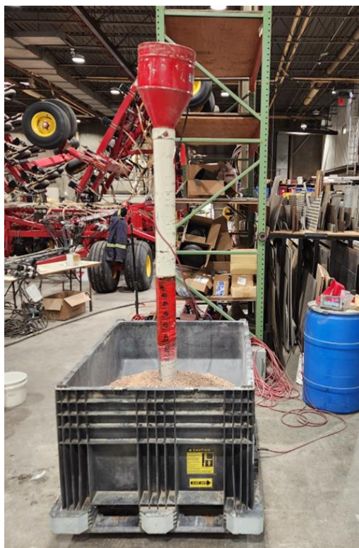
Figure 1. Aeration tube placed in plastic tote of pinto beans to condition product to appropriate moisture level for testing.
