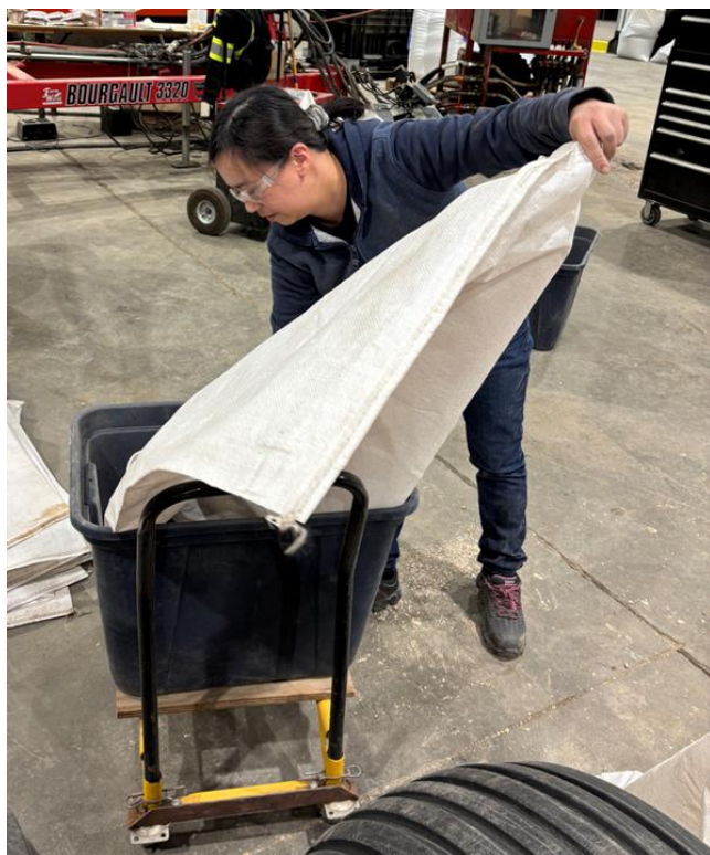
Figure 7. Collection bag being carefully emptied into a plastic tote to ensure appropriate mixing prior to sampling.
