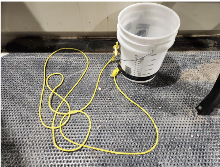
Figure 5. 20-L (5-gallon) pail suspended with ropes (left) and filled with bean seeds being carefully lowered into the air cart to prevent any bean seed damage (right).
