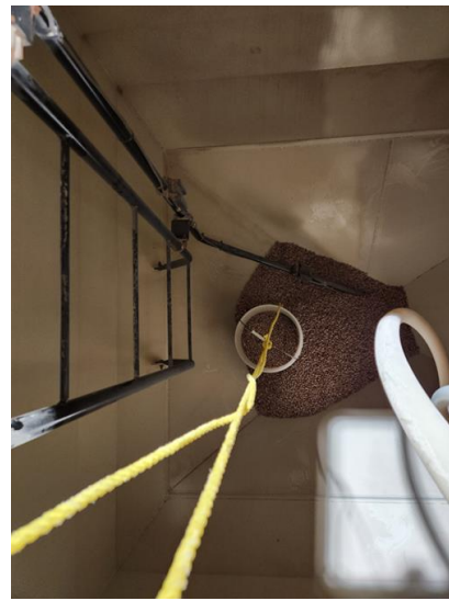
Figure 5. 20-L (5-gallon) pail suspended with ropes (left) and filled with bean seeds being carefully lowered into the air cart to prevent any bean seed damage (right).
