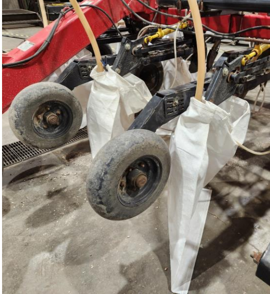
Figure 6. Bags clamped on individual openers to capture seed during testing.
