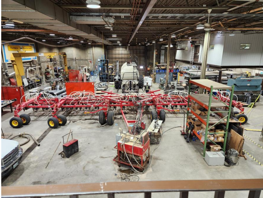
Figure 4. Bourgault PHD 3320-10 toolbar with 6550ST air cart assembled in PAMI shop for testing.
