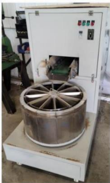
Figure 5. Rotary sampler with 12-Bin drum.
