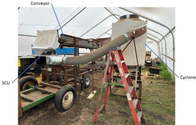
Figure 2. SCU test stand configuration
