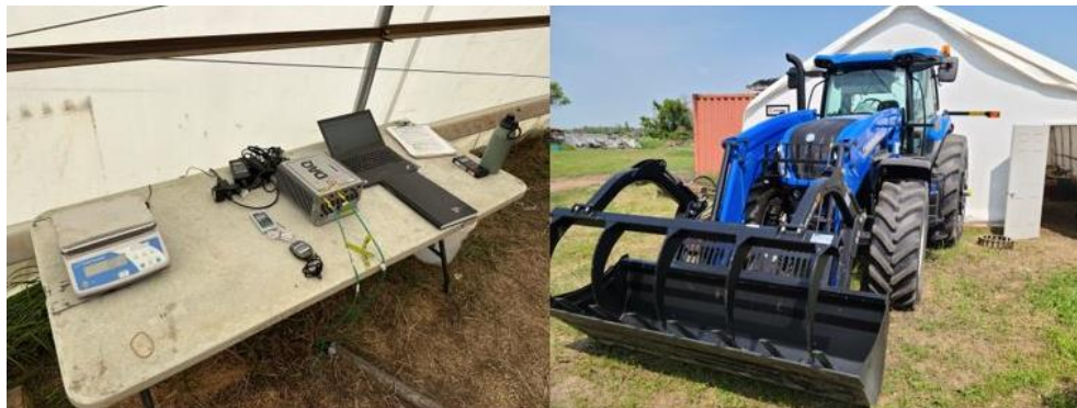
Figure 3. SCU test stand data acquisition and tractor unit (New Holland T7.230).
