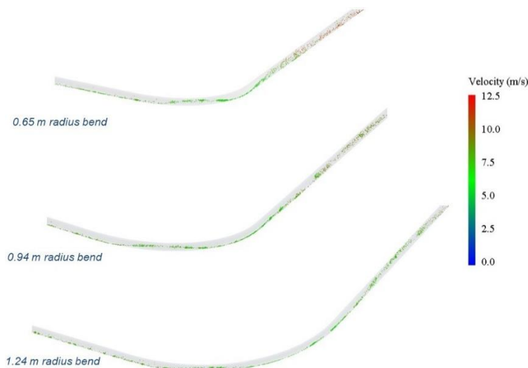
Figure 12. 90° bend simulations with velocity gradient profiles (0 to 12.5 m/s).
