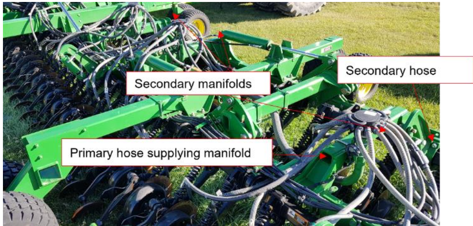
Figure 2. Secondary manifolds located on the air drill frame. The division of product and air occurs passively in the secondary manifold.
