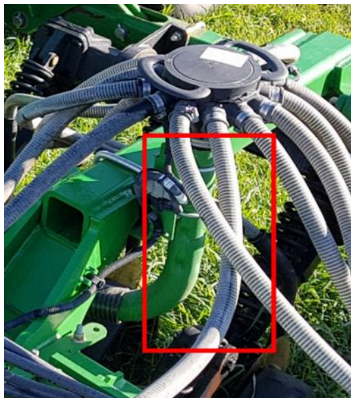
Figure 3. J-tube transitioning from nominally horizontal flexible secondary hose to the secondary distributor which is fed from the underside.
