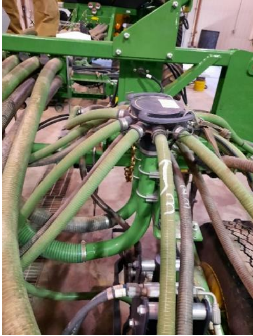
Figure 12. The primary hose geometry leading to distributor 3. Distributor 4 had similar geometry.
