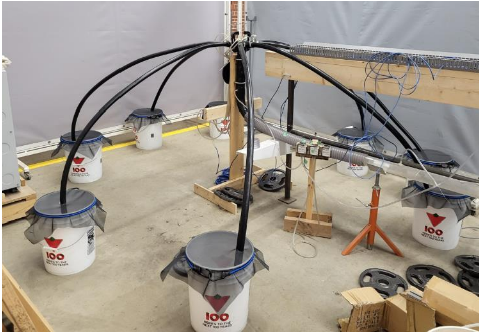
Figure 31. The distributor and secondary hose setup used in the lab-scale testing at the University of Saskatchewan Air-Handling Laboratory. Equal-length secondary hoses are shown in this image. Credit: Sarita Victoria Casas Urrunaga.
