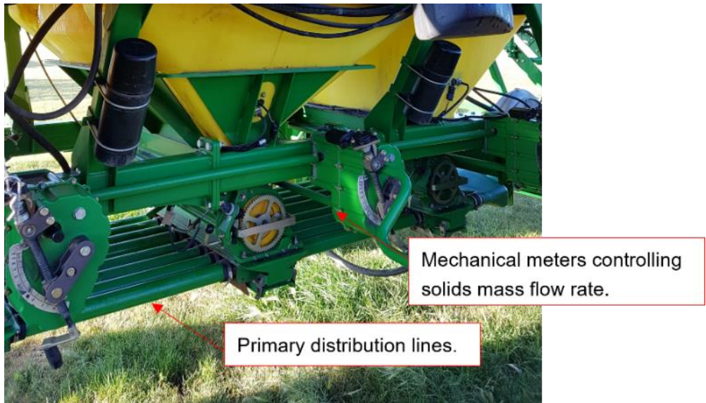
Figure 1. Primary meters controlling mass flow rate of solid product into primary distribution hoses.
