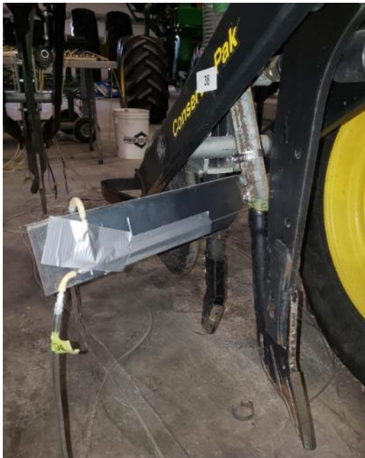
Figure 17. A pitot-static tube installed at a row unit downstream of distributor 4 or 6.
