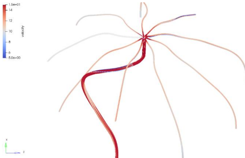
Figure 49. Streamlines upstream of distributor 6 simulated at 2,200 RPM.
