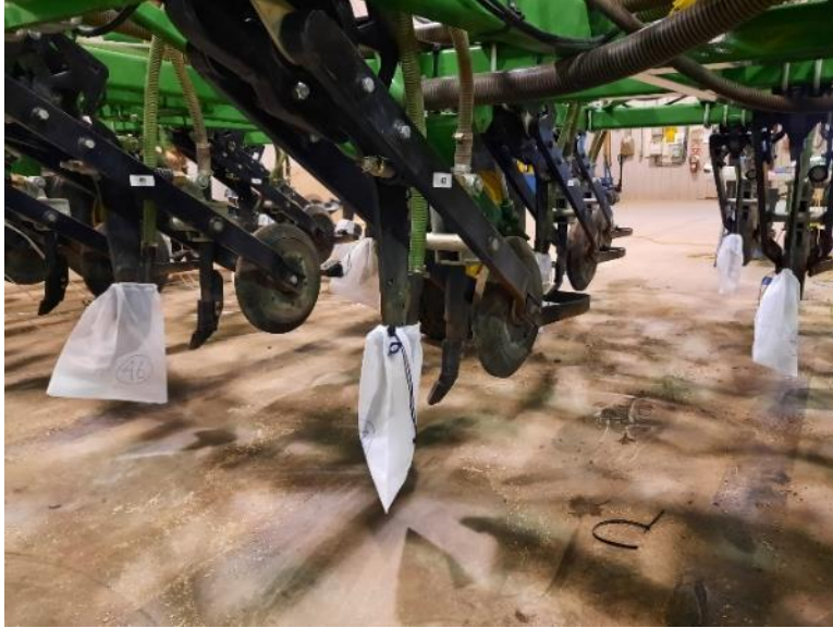
Figure 14. Numbered mesh bags fastened to each row unit to capture the canola distribution.
