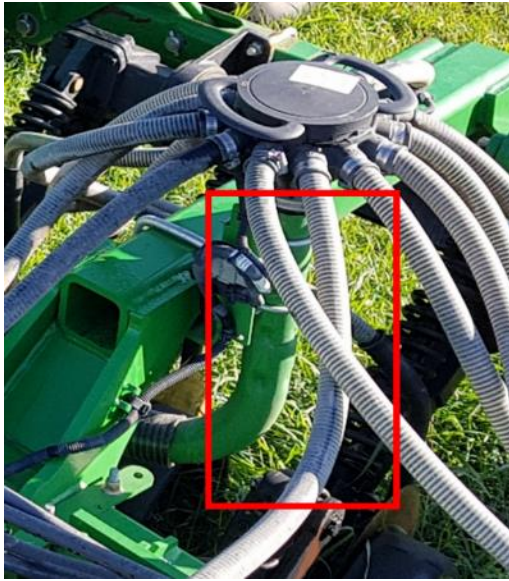
Figure 3. J-tube transitioning from nominally horizontal flexible secondary hose to the secondary distributor which is fed from the underside.
