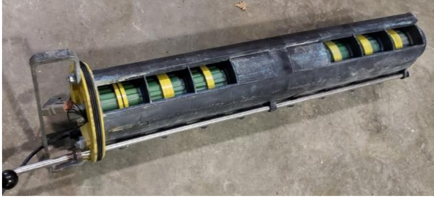
Figure 8. The meter roller used for canola testing, as specified by the manufacturer.
