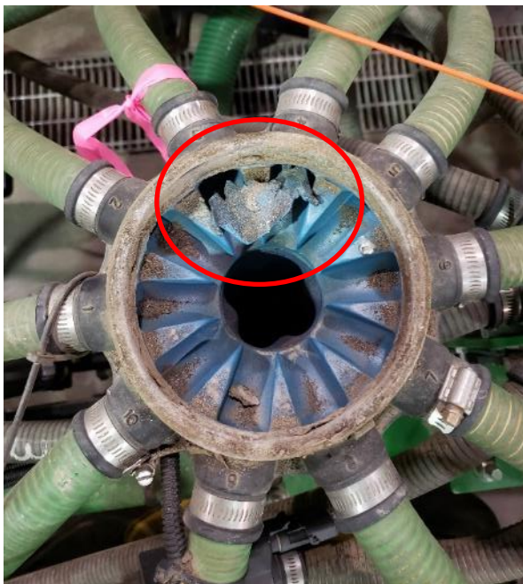
Figure 19. Debris found in distributor 3 at the conclusion of testing, partially blocking outlets 1 and 2.
