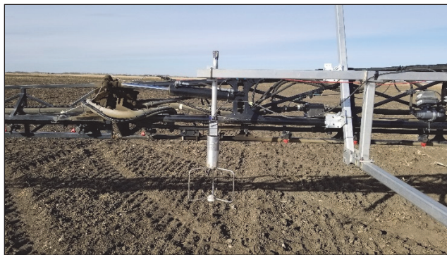
Figure 11. Position of ultrasonic anemometer laterally located at 8.30 m in the Far Boom measurement region. The anemometer is shown while measuring below the nozzle plane.
