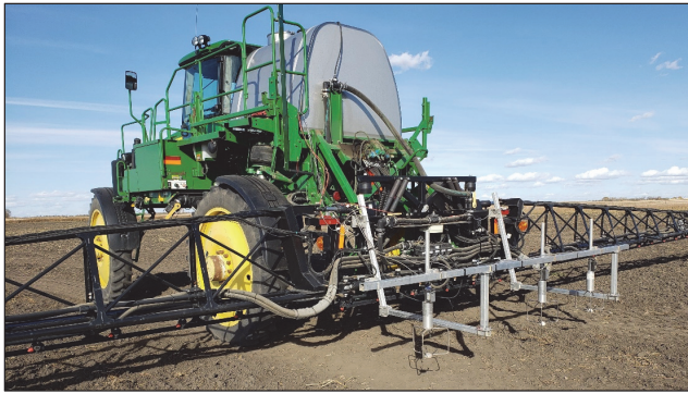
Figure 2. Aluminum frame used to mount three anemometers on the boom, shown in the Behind Tractor configuration. The anemometers were oriented upside down in this measurement region.
