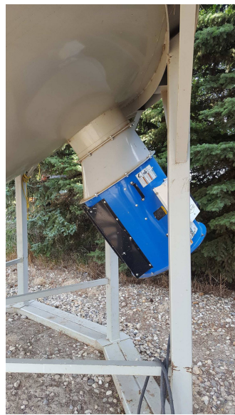
Loading peas into the 15 bu test bins at PAMI's Humboldt facility (left), Fan and transition duct used for one of the bin-scale airflow assessments with a partner producer (center), Unloading lentils from the 15 bu test bins at the end of the lentil drying trial (right).
