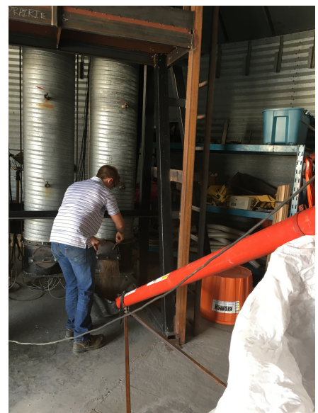
Loading peas into the 15 bu test bins at PAMI's Humboldt facility (left), Fan and transition duct used for one of the bin-scale airflow assessments with a partner producer (center), Unloading lentils from the 15 bu test bins at the end of the lentil drying trial (right).
