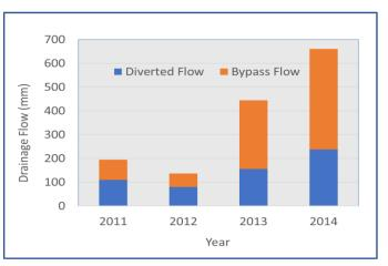
Figure 4. Flow diverted to riparian zone (buffer strip vs flow bypassing riparian zone at Bear Creek (Iowa) (Jaynes et al.; ADMC website).
