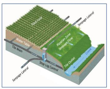
Figure 2. Plan view of saturated buffer, including stop log control structure, seepage lateral and riparian zone parallel to the outlet waterway (source: modified from TransformingDrainage.Org).
