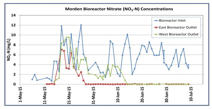
Figure 3. Reduction in NO<sub>3</sub>-N Concentration – Bioreactor (Agriculture and Agri-Food Canada, Unpublished).
