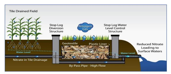
Figure 2. Illustration of woodchip bioreactor components/processes (modified from original on Ag Web by Farm Journal, 2012).
