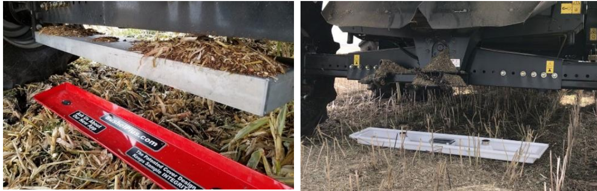
Figure 2. Drops pans used to measure losses. a) Bushel Plus b) Schergain. Images sourced and adapted from (Bushel Plus, n.d.) and (Schergain n.d.).
