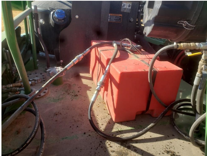
Figure 3. Marine auxiliary tank on John Deere X9 1100 combine.
