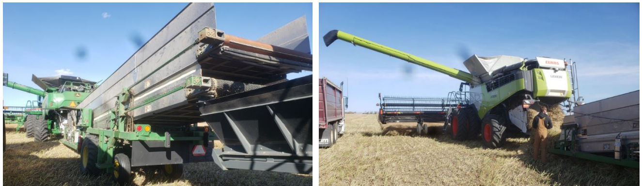
Figure 1. John Deere X9 (left) and CLAAS Lexion 8800 (right) attached to collector during loss curve testing.
