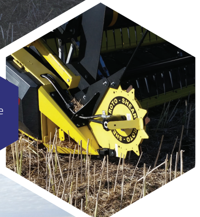
Figure 15. Vertical Knife Divider
