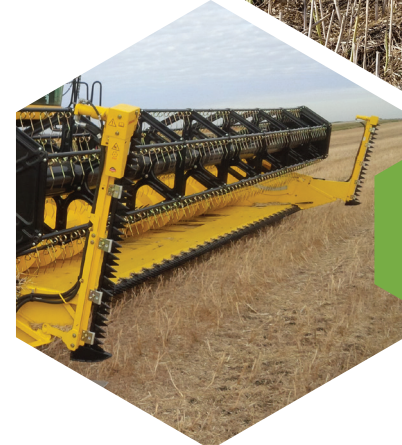
Figure 14. Rotary Knife Divider
