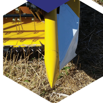
Figures 22. Plastic dividers to ease divider transition
