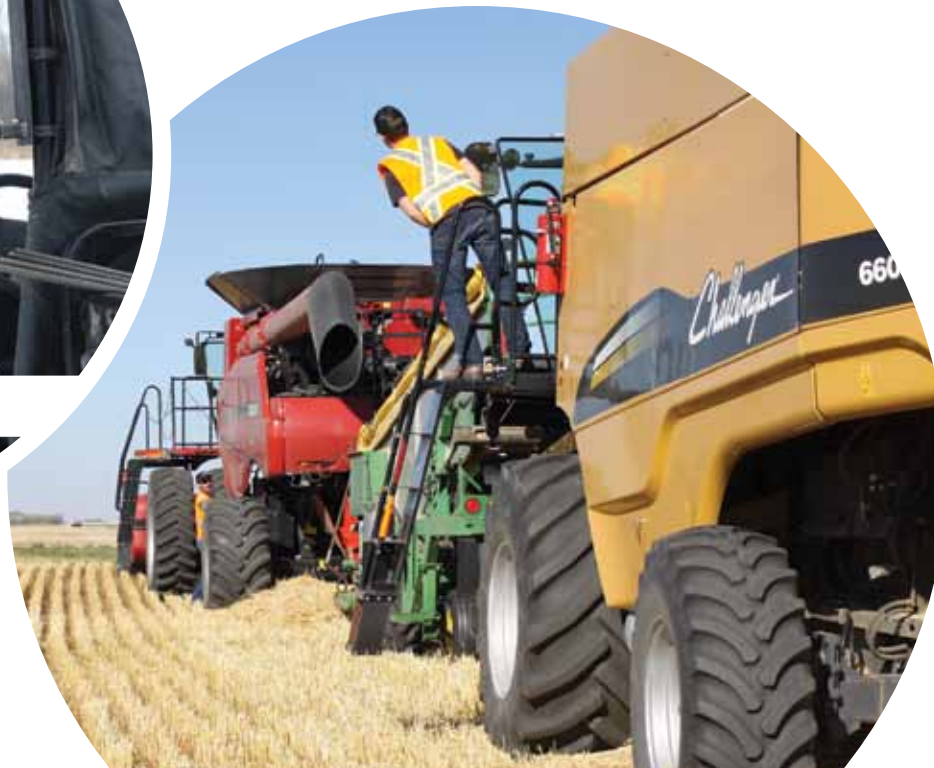
combine testing evaluating grain loss monitor sensitivity
