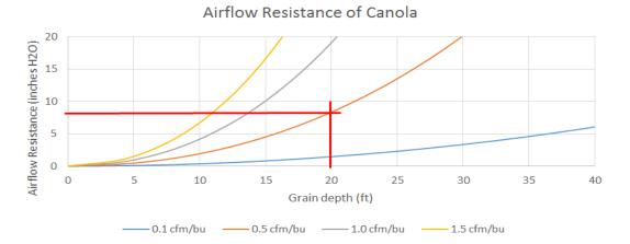
Figure 2. Estimated airflow resistance (static pressure) for canola.
