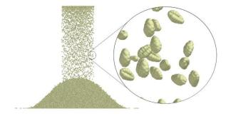
DEM considers a system as a collection of discrete entities; this is in contrast to the Finite Element Method (FEM) which treats a bulk particulate system as a continuum. Therefore DEM provides knowledge of the particle behaviour at the scale, enabling a better prediction and understanding of the macro scale (the bulk
