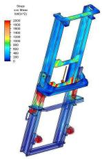
FEA has become an everyday tool that supports the design process. Linear FEA with static loads is frequently used and covers a broad range of the situations encountered by design engineers. When larger deformation are involved, nonlinear analysis need to be performed to accurately predict the behaviour of the system.
