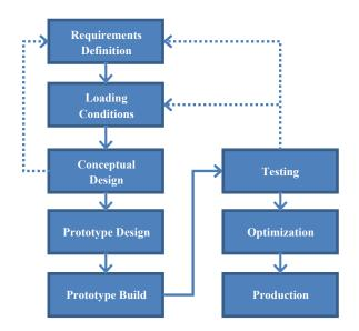
When the conceptual design has reached a sufficient level of details, it has become the prototype design that can be built or implemented. At that point a testing regime can be contemplated and with test results, the design can be improved or optimize to finally reach a level that satisfies production requirements. Now let's look at where modeling and simulation can be used in the design cycle.
