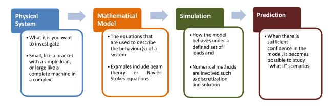
**Model**: Mathematical representation (object) that has the ability to predict the behaviour of a real system under a set of defined operating conditions and simplifying assumptions. Those mathematical representation are derived in a number of ways.
