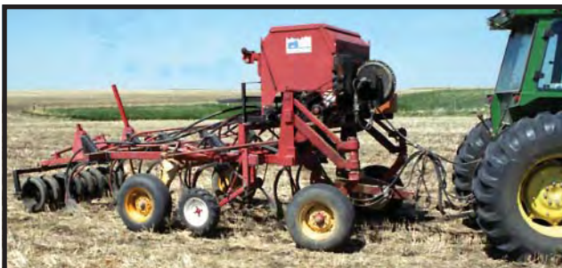
Figure 2. The other air-seeder is an 8 ft (2.4 m) wide floating hitch cultivator. The cultivator has 4 rows of 8 C-shanks with 12 in (305 mm) spacing. A Gandy air pneumatic seed/fertilizer metering applicator system is mounted above the cultivator frame. The Gandy material box is split in half for seed and fertilizer. A gang packer mounted at the rear of the cultivator provides on-row packing.
