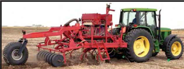
Figure 1. One air-seeder is a 3-point hitch mount with a large rear support wheel. The seeder is 10 ft (2.8 m) wide and is made up of two frames. The main frame supports the material tanks and delivery system. There are four seed and fertilizer tanks that use an electric driven and monitored fluted metering system. The material is delivered to the openers using a pneumatic venturi system. There are air delivery material blockage sensors in each hose. The second frame is a sub frame that is interchangeable to the main frame. There are several sub frames constructed which are designed to accommodate different types of shanks with different mounts and spacings. Eight to ten shanks can be mounted on the sub frames. There are different widths of gang packers available that mount to the rear of the sub frame for on-row packing if required. The sub frames are easily changed in the field.
