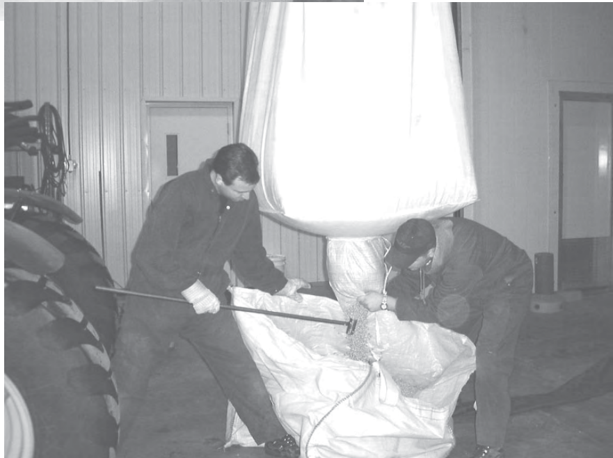
Collecting a check sample for comparison with chickpea samples that have been through the air seeder.
