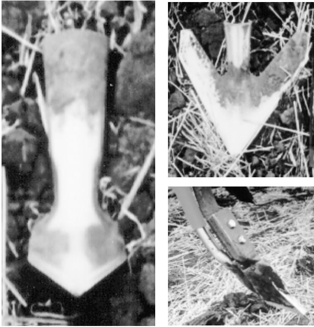
Clockwise, from top left: Spoon, Sweep, Knife. PAMI applied rates of 0, 35, 70 and 105 pounds (7.7, 15.4, 23.1 kg), respectively, of N as urea with the seed on 8" centres. Seed and N were spread 3/4 inches (19 mm) with a knife, 2 inches (50 mm) with a spoon, and 7 inches (175 mm) with an 8 inch (200 mm) sweep. Preliminary results suggest the knife presents the most risk to emergence damage and yield loss, and the sweep the least. Note: Spread width is not usually the same width as the opener. PAMI used a special spreader boot and a high fan speed to achieve the wide spread pattern with the sweep.
