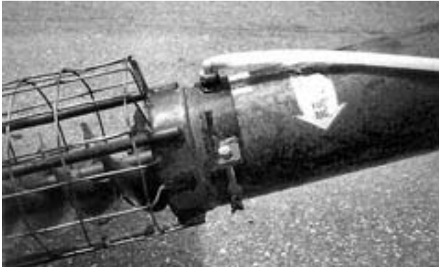
FIGURE 6. Liquid Outlet into Grain Stream.
