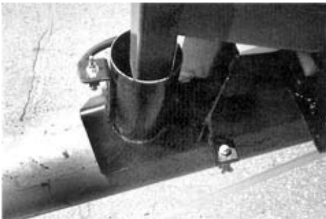
FIGURE 2. Port in Auger Tube.
