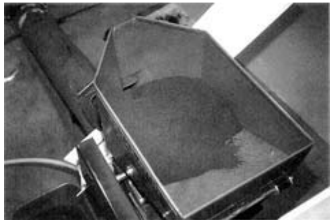
FIGURE 4. Sticking Inoculant in Hopper.
