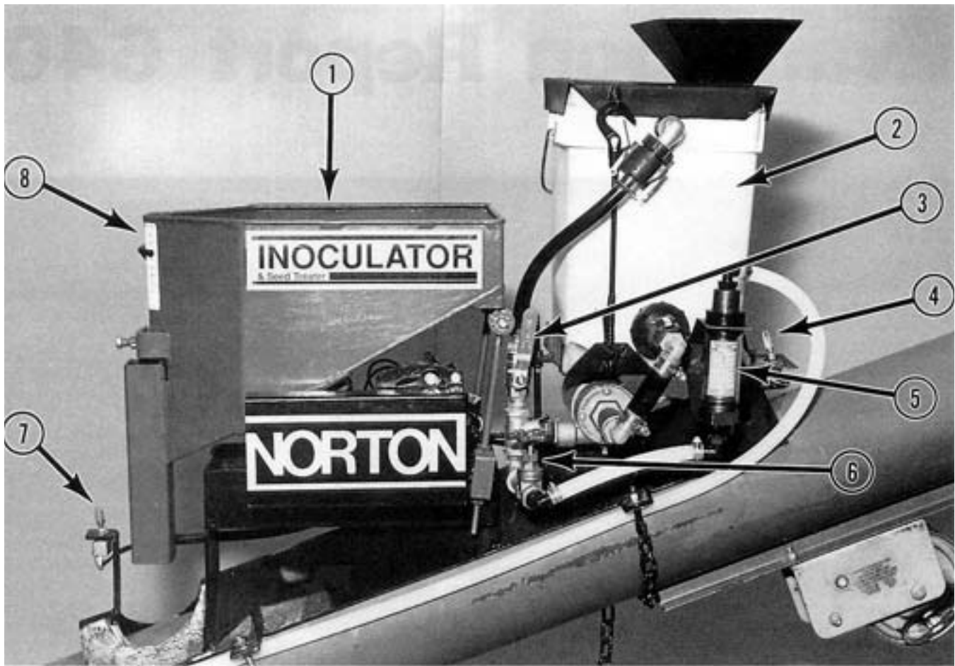
FIGURE 1. Norton Inoculator/Seed Treater: (1) Inoculant Hopper, (2) Liquid Tank, (3) Return Valve, (4) Pump Switch, (5) Liquid Flow Meter, (6) Flow Control Valve, (7) Shaker Switch, (8) Inoculant Hopper Gate.
