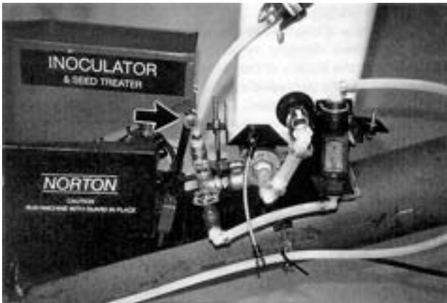
FIGURE 7. Interference Between Hopper and Return Line when Adjusting for Steep Auger Angles.
