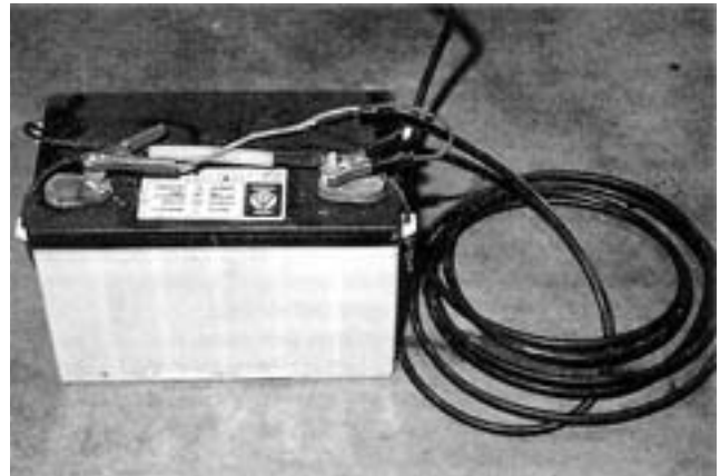
FIGURE 9. 12 Volt Power Hook-up.
