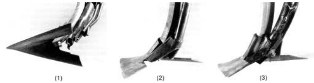
FIGURE 13. Air Seeder Boots: (1) Rearward Deflecting, (2) Forward Y-Dividing, (3) Forward Full Spreading.
