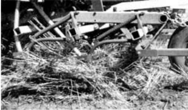
FIGURE 15. Trash Plugging in a Hoe Drill.
