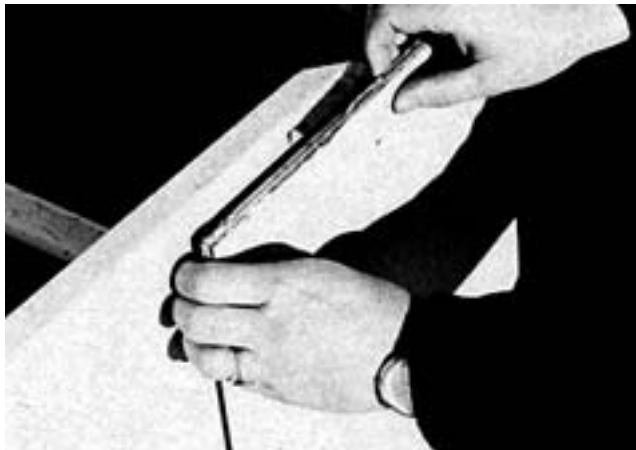
FIGURE 7. Pinch Points on Seed Hopper Extension.
