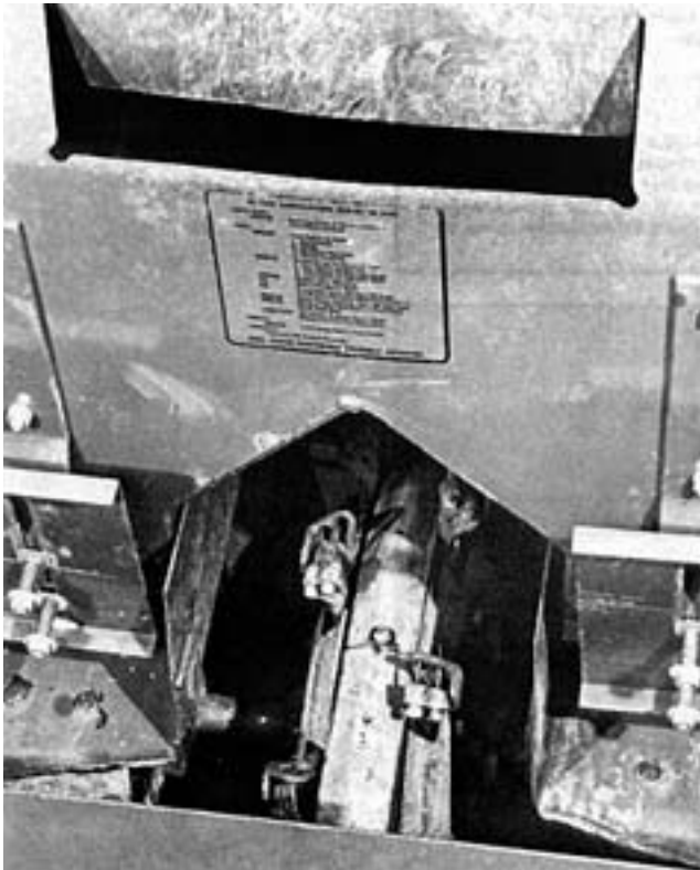
FIGURE 4. Access Holes Cut in the Seed Hopper.
