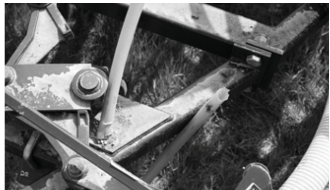
Figure 18. Damage to Secondary Hose by Depth Linkage System.
