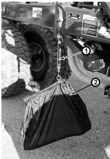
Figure 17. Rate Calibration: (1) Spring Scale and (2) Rate Check Bag.
