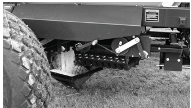
Figure 13. Unloading Material from Flexi-coil Tank.
