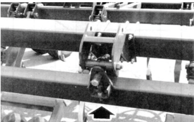
FIGURE 10. A Levelling Adjustment for the Back of the Drill.
