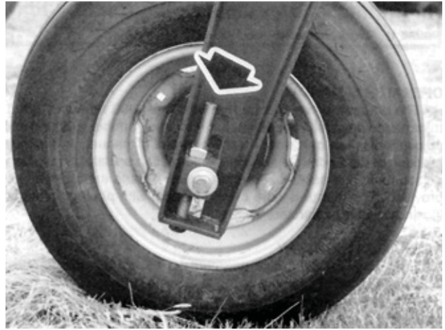
FIGURE 11. Levelling Adjustment on the Wing Section Front Castor.
