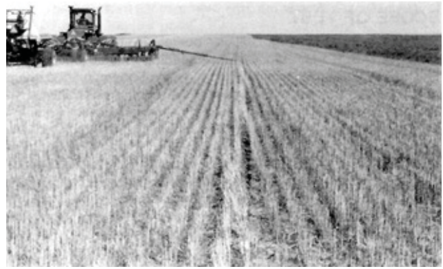
FIGURE 7. Mark Left by Till Mark Endmarker in an Untilled Field.
