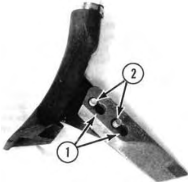
FIGURE 5. (1) Lower Holes Used for 43 Degree Shank (2) Upper Holes Used for 50 Degree Shank.
