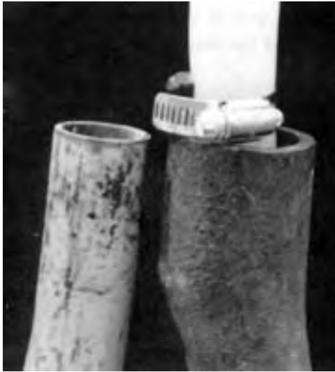
FIGURE 4. Connection of Delivery Hose to Seed Boot.
