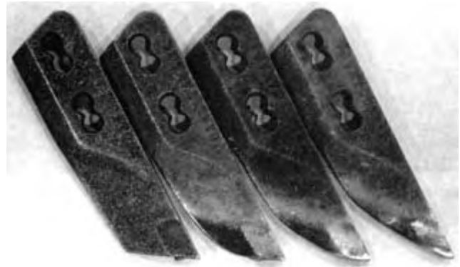
FIGURE 6. Wear on the Banding Knives After 20 ac (8 ha) per Knife, 30 ac (12 ha) per Knife and at the End of the Test.
