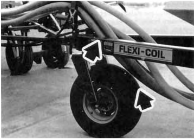
FIGURE 21. Interference at Front Pivot Point.
