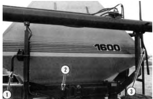
FIGURE 14. Auger in Transport Position: (1) Front Look Arm, (2) Front Pivot Arm (3)Rear Lock Handle.
