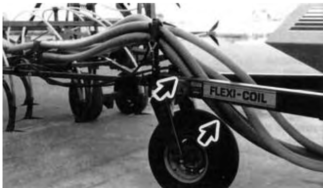
FIGURE 17. Interference at Front Pivot Point.
