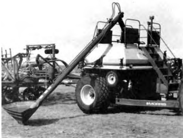
FIGURE 12. Fill Position of Auger.
