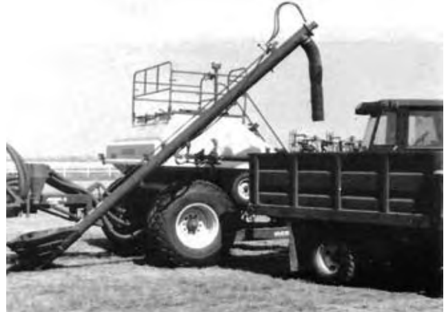
FIGURE 15. Using Clean-Out System.
