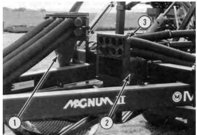
FIGURE 14. (1) Cyclone, (2) Sample Collector, (3) Air Seeder Distribution.
