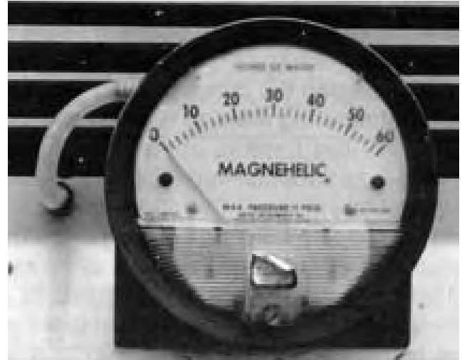
FIGURE 19. System Pressure Gauge.
