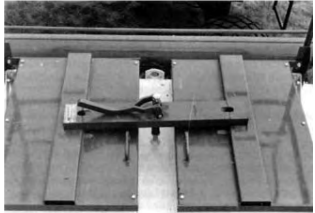
FIGURE 13. Tank Lids and Latches.
