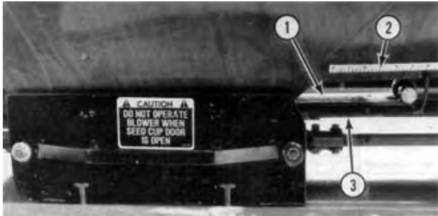
FIGURE 20. Application Rate Adjustment: (1) Meter Door, (2) Gate Opening Scale, (3) Flow Control.
