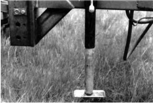
FIGURE 17. Inadequate Lifting Height of Hitch Jack.
