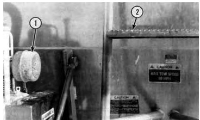
FIGURE 21. (1) Engine Exhaust, (2) Applicator Ladder.
