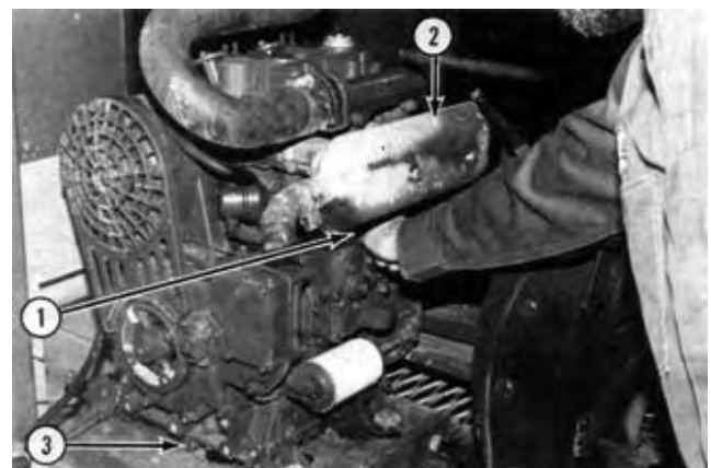
FIGURE 21. (1) Engine Throttle and Shut-off, (2) Exhaust, (3) Oil Drain Plug.
