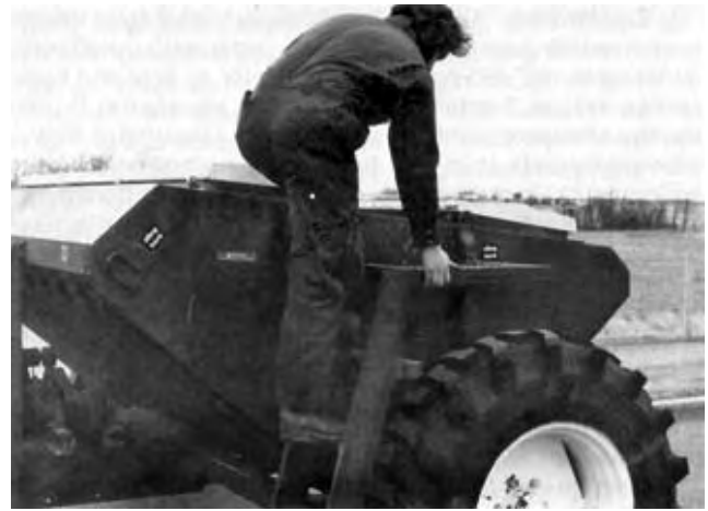
FIGURE 19. Tank Access Ladder.
