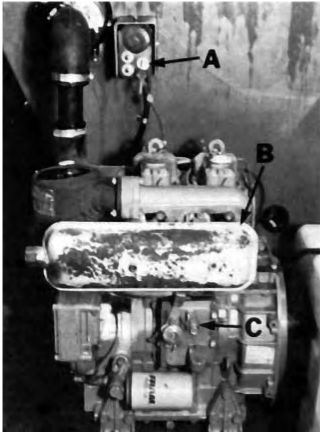
FIGURE 18. (A) Engine Ignition, (B) Engine Exhaust (C) Engine Fuel Shut Off.
