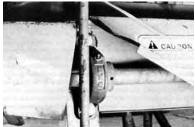
FIGURE 15. Poor Access to Grease Fittings behind Power Take-off Shield.
