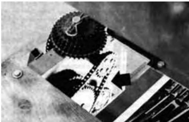
FIGURE 17. Poor Accessibility of High-Low Range Sprockets.
