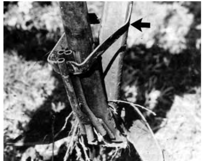
FIGURE 19. Damaged Seed Boot Clamps.
