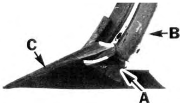
FIGURE 9. Friggstad Seed Boot: (A) V-shaped De flector, (B) Seed Boot, (C) Sweep.
