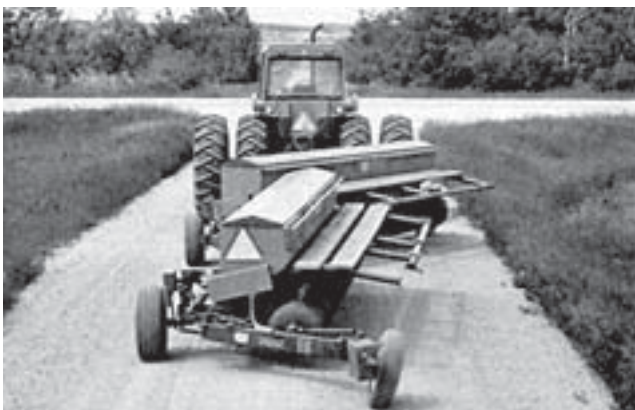
FIGURE 13. Semi-Transport Position with Hitch Brace Collapsed.
