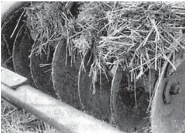
FIGURE 13. Trash and Mud Buildup Between the Scrapers and Disks.
