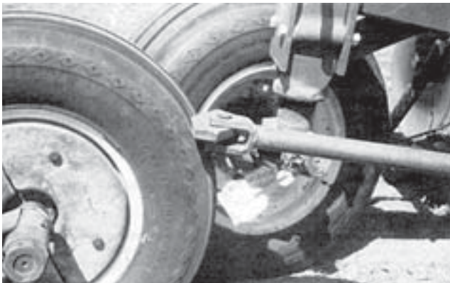
FIGURE 17. Interference Between Furrow Wheel Steering Arm and Rear Furrow Wheel when Placing into Full Transport with the Disk Gangs Raised.
