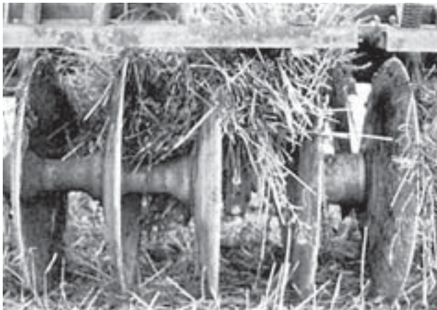
FIGURE 13. Trash and Mud Buildup Between the Disks and the Disk Gang Arm.
