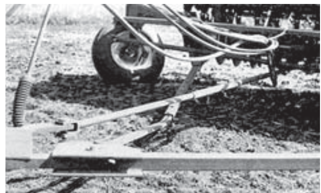
FIGURE 21. Buckled Hitch Brace.
