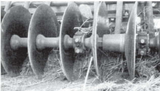
FIGURE 14. Small Rock Jammed Between the Disk and Disk Gang Arm.
