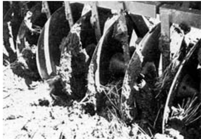
FIGURE 11. Mud Buildup on Disks when Operating in Wet Fields.
