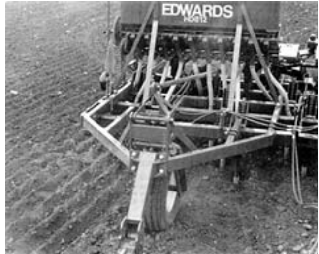
FIGURE 17. Poor Visibility of Far Right Shank from Tractor.
