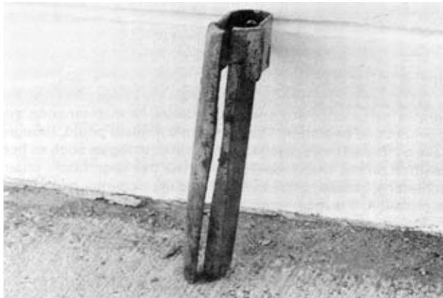
FIGURE 20. Broken Hoe Opener.
