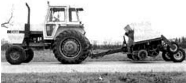
FIGURE 9. Ground Clearance During Transport.
