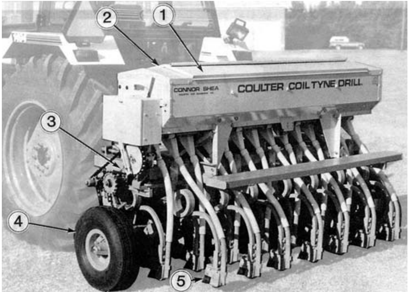
FIGURE 1. Connor Shea Coil Tyne Coulter Drill: (1) Fertilizer Box, (2) Seed Box, (3) Drive Mechanism, (4) Depth Wheel, (5) Hoe Opener.
