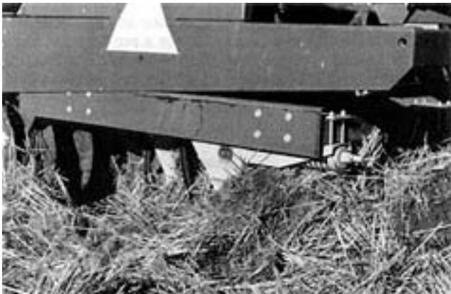
FIGURE 6. Plugged Hoe Opener Drill in Wet Wheat Stubble Condition.
