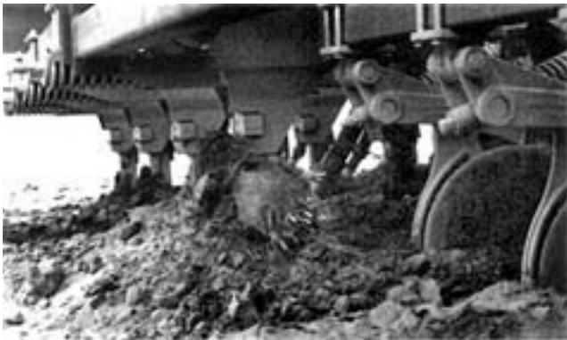
FIGURE 5. Straw Wrapped Around Hoe Opener.
