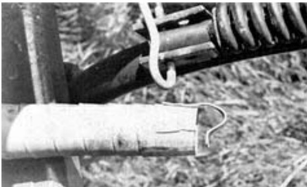
FIGURE 23. Seed Tube Connection Failure.
