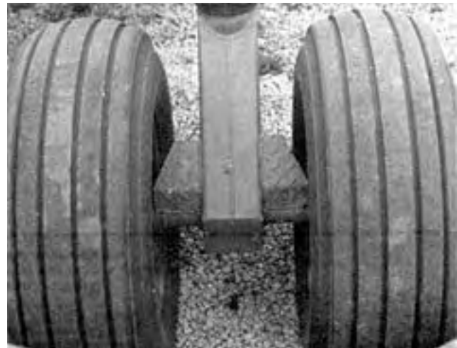
FIGURE 1. Castor Wheels With Reinforcements.
