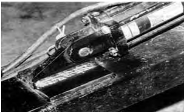
FIGURE 12. Rewelded Cylinder Lug.
