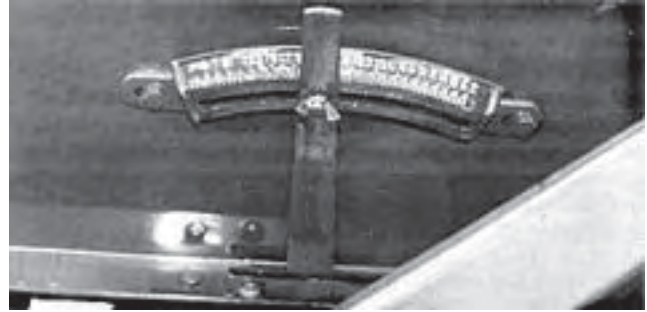
FIGURE 14. Seeding Rate Selection Lever.
