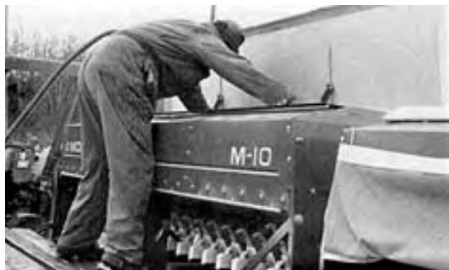
FIGURE 12. Difficult Closing of the Grain and Fertilizer Box Lids.
