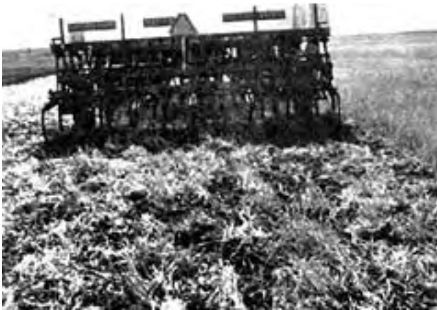
FIGURE 6. Heavy Trash Cleared by Morris 80-14 on Wheat Stubble not Tilled Immediately Prior to Seeding.
