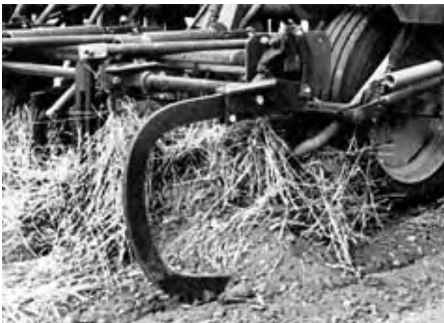
FIGURE 7. Plugging near Wheel in Pre-Tilled Fields.
