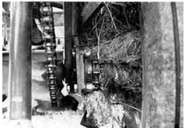
FIGURE 15. Flax Straw Wrapped around Chain Drives.
