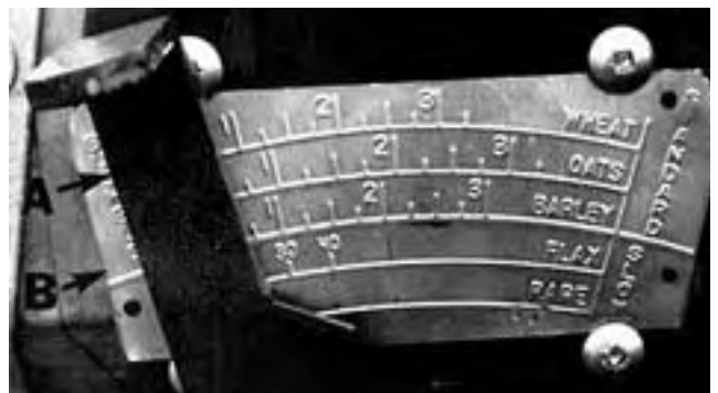
FIGURE 10. Seed Rate Control: (A) Lever, (B) Indicator Plate.
