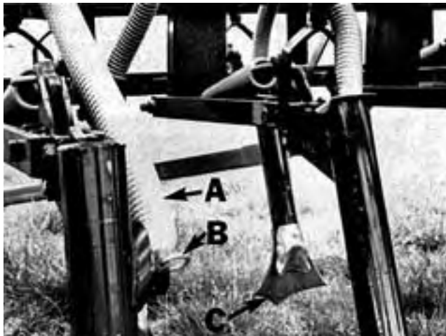
FIGURE 12. Rear Grain Tube: (A) Flexible Grain Tube, (B) Hair Pin Clip, (C) Opener Tube.
