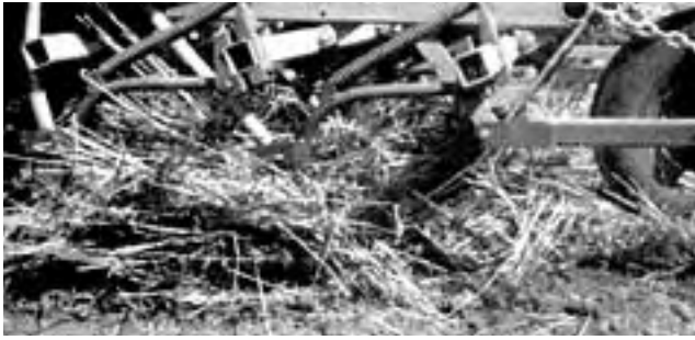
FIGURE 5. Long Straw Collecting around Hoe Shanks.
