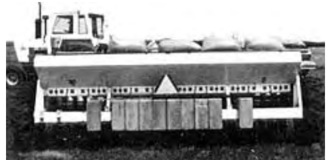
FIGURE 3. Concrete Ballast Blocks Added to Drill Frame.
