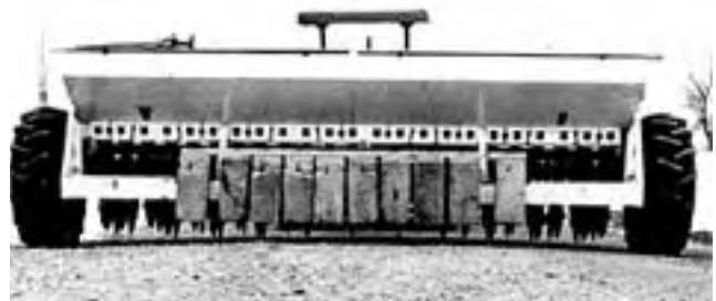
FIGURE 18. Limited Opener Clearance When Transporting.
