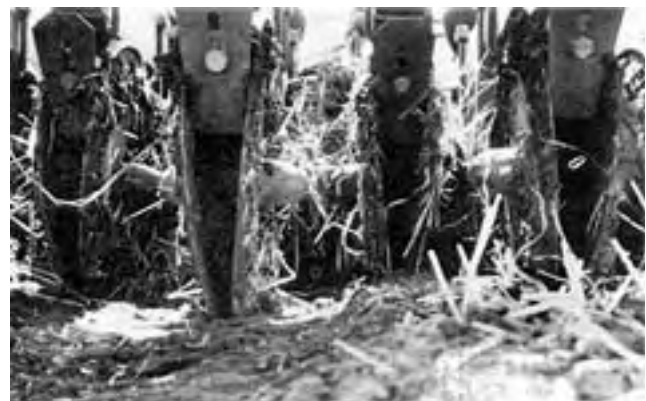
FIGURE 14. Mud Buildup on the Cutting Coulters and Double Disks.
